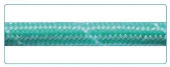
A double braided rope that has a polyethylene outer cover and a polyamide internal core. The outer polyethylene braided construction gives it firmness without taking it the necessary smoothness and flexibility for a good handling, preventing entanglement and allowing higher protection and adjustment of PE/PA Stripe ropes, reducing assembly time and on board repairing.
