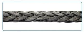
Made from HMWPE fibres and protected by a self unique impregnation that improves its abrasion resistance, Cotesi D-tech ropes must be considered when high breaking strengths are required. Using a torque free 12 strands bright and construction, D-tech is seven times stronger than steel wire of same weight and has proven to be a cost-saving replacement for wire rope in several applications.
