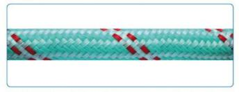
A double braided rope that has a polyethylene outer cover and an internal core of polyamide and lead for faster sinking. The outer polyethylene braided construction gives it firmness without taking it the necessary smoothness and flexibility for a good handling, preventing entanglement and allowing higher protection and adjustment of PE/PA Stripe ropes, reducing assembly time and on board repairing.
