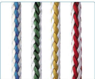
A 12 strands high tenacity braided polyamide rope specially designed for pelagic nets and with identification colours for better handling of the trawl, that don't fade in use. Its self unique coating gives it firmness and increases its wear and abrasion resistance.
