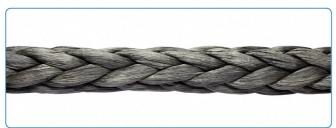
Made from HMWPE fibres and protected by a self unique impregnation that improves its abrasion resistance, Cotesi D-tech ropes must be considered when high breaking strengths are required. Using a torque free 12 strands braided construction, D-tech is seven times stronger than steel wire of same weight and has proven to be a cost-saving replacement for wire rope in several applications.
